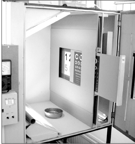
Figure 1: The purpose-built viewing chamber (access panels shown open)
