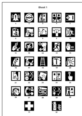
Figure 4 A typical symbol matrix used for the mutual confusion test
