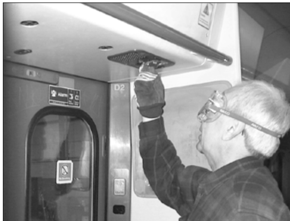
Figure 6 User trials underway with the Passenger Alarm device in the rail vehicle
